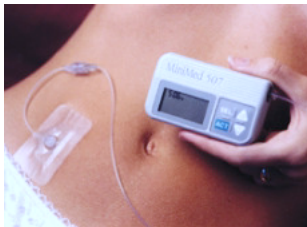
Fig. 1. Device for the continuous infusion of subcutaneous prostacycline (treprostinil) with the insertion point in the abdominal wall (MiniMed Pump 507).
