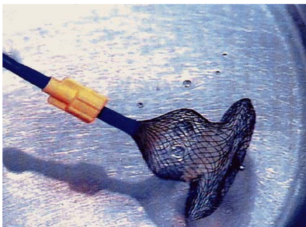
Fig. 2. Liberation of bubbles upon extracting the device from the sheath after the first introduction of same.
